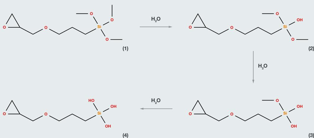
The reaction steps are strongly pH-dependent. Complete hydrolysis in neutral medium at room temperature takes about 24 hours. The starting compound GLYMO can be detected for about eight hours. The last reaction step, i.e. the opening of the epoxy ring to trihydroxyglycol, is much slower. A complete reaction can only be expected after a storage period of more than one month. In acidic solution
